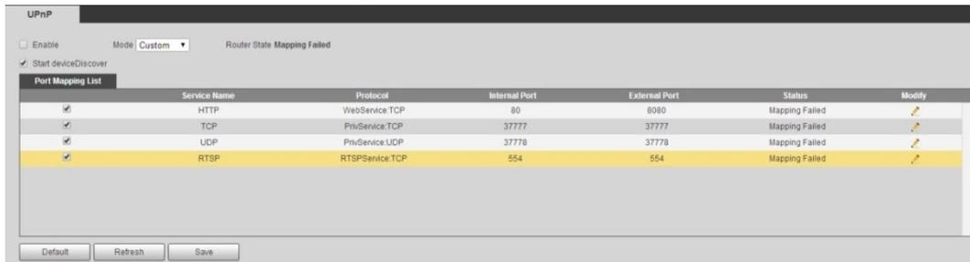
**Step 2** Select the **Enable** check box, and there are two mapping modes: **Custom** and **Default**.
