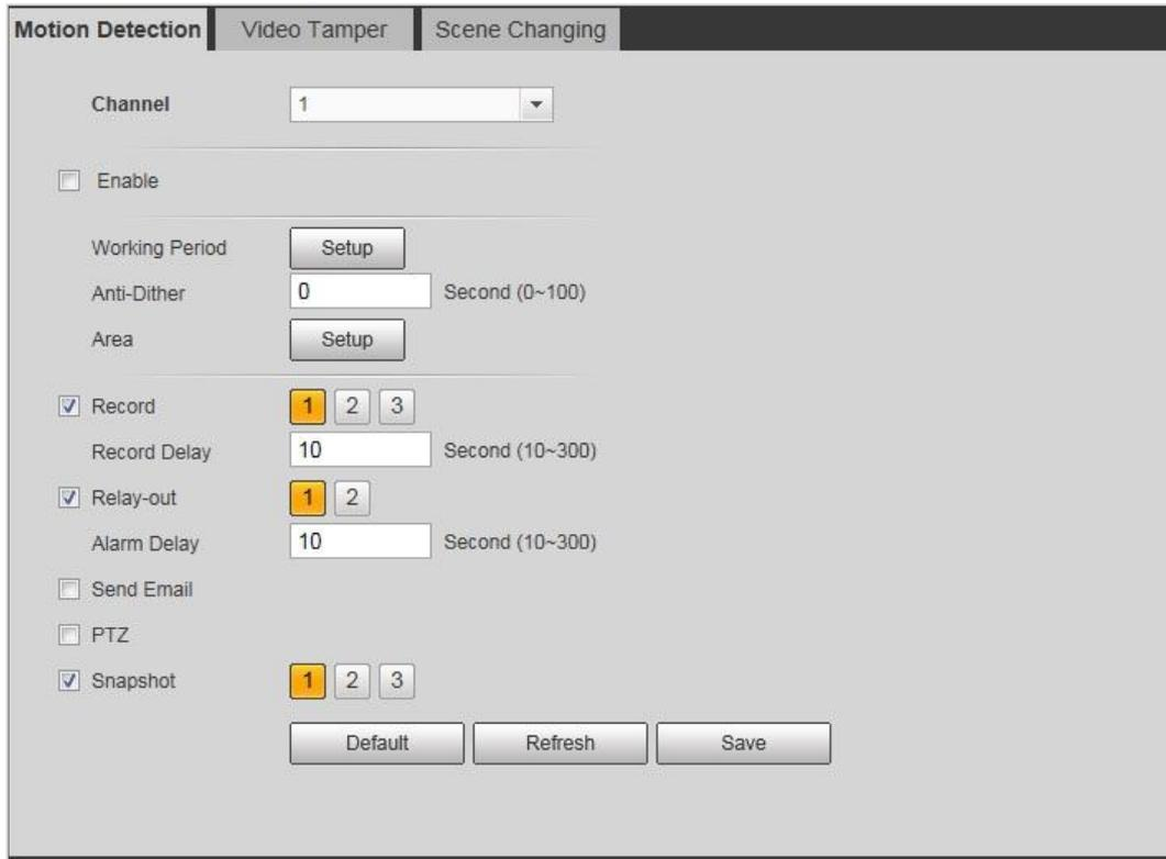
**Step 2** Select the **Enable** check box to enable motion detection.
