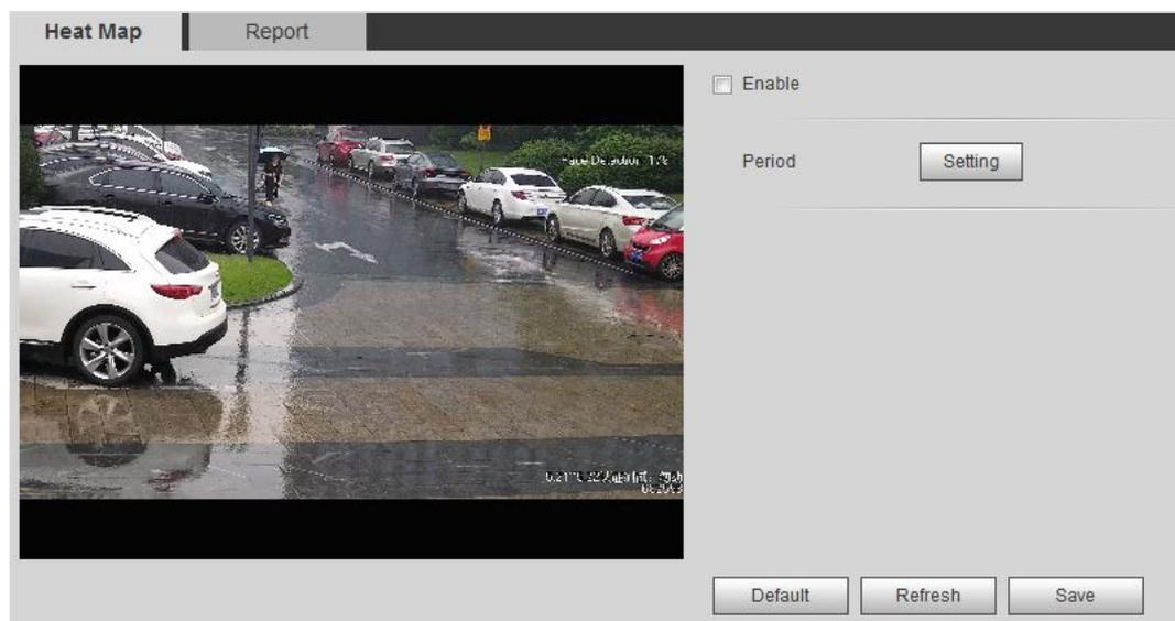
**Step 2** Select **Enable** to enable the heat map function.
