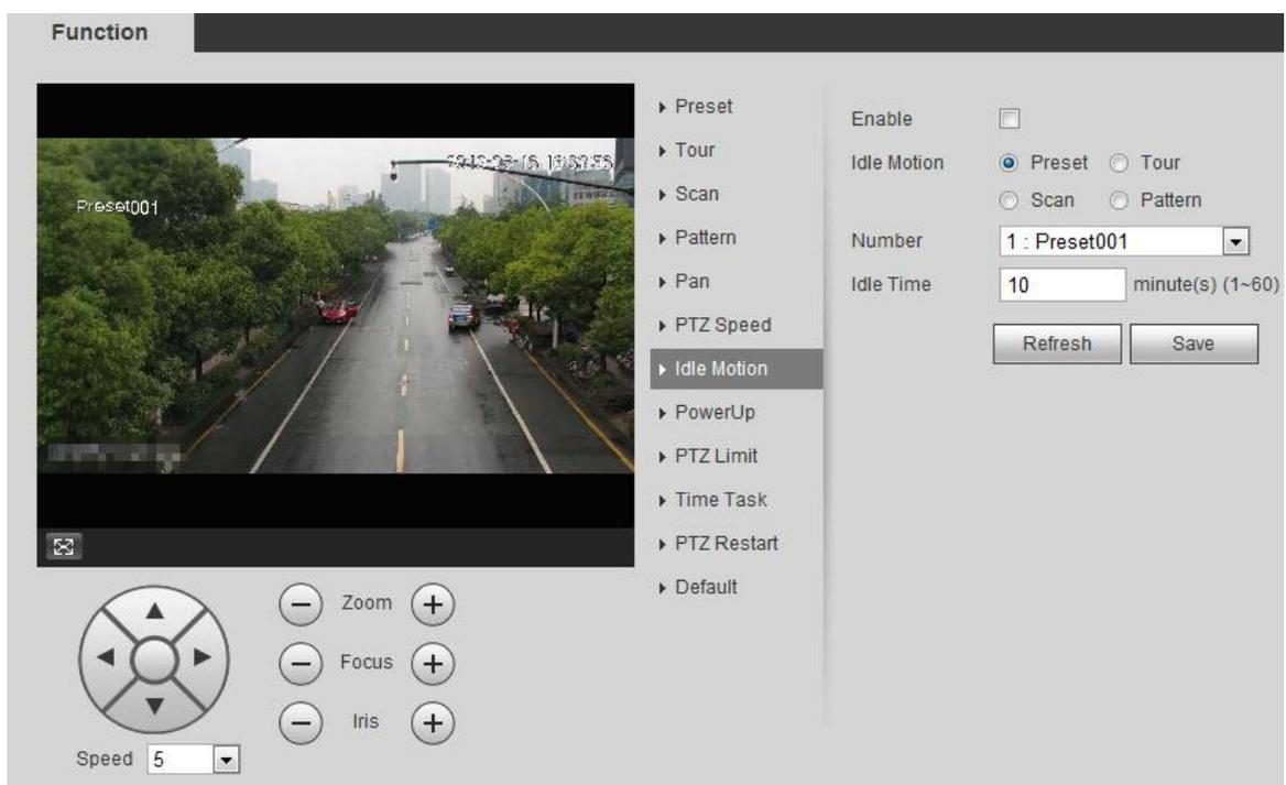
**Step 2** Select the **Enable** check box to enable idle motion.
