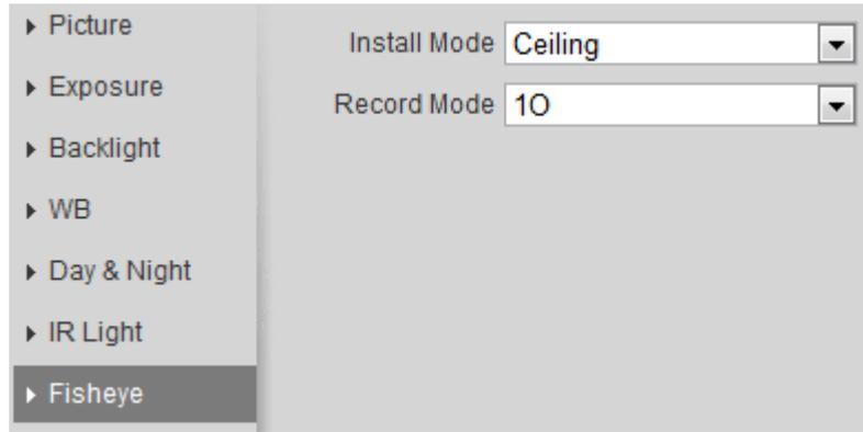
Step 2 Set install mode and record mode. For details, see Table 4-16.
