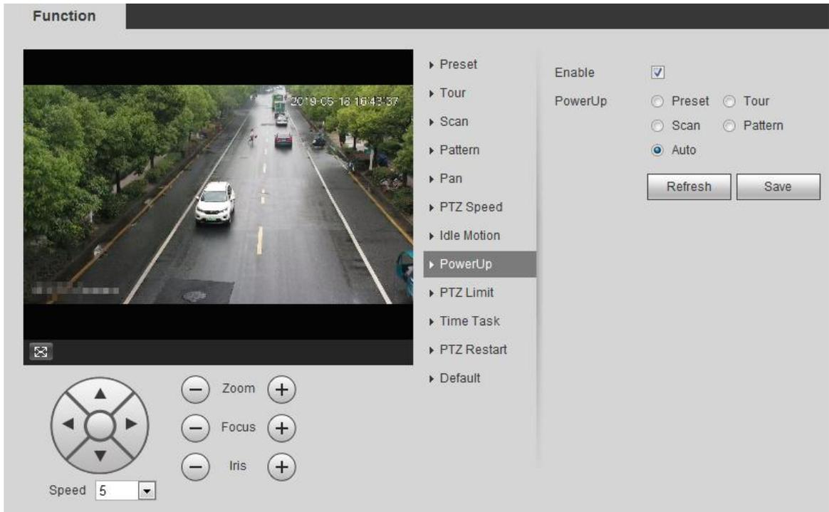
**Step 2** Select the **Enable** check box to enable powerup motion.
