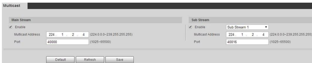
**Step 2** Select the **Enable** check box, and enter IP address and port number. For details, see Table 4-28.
