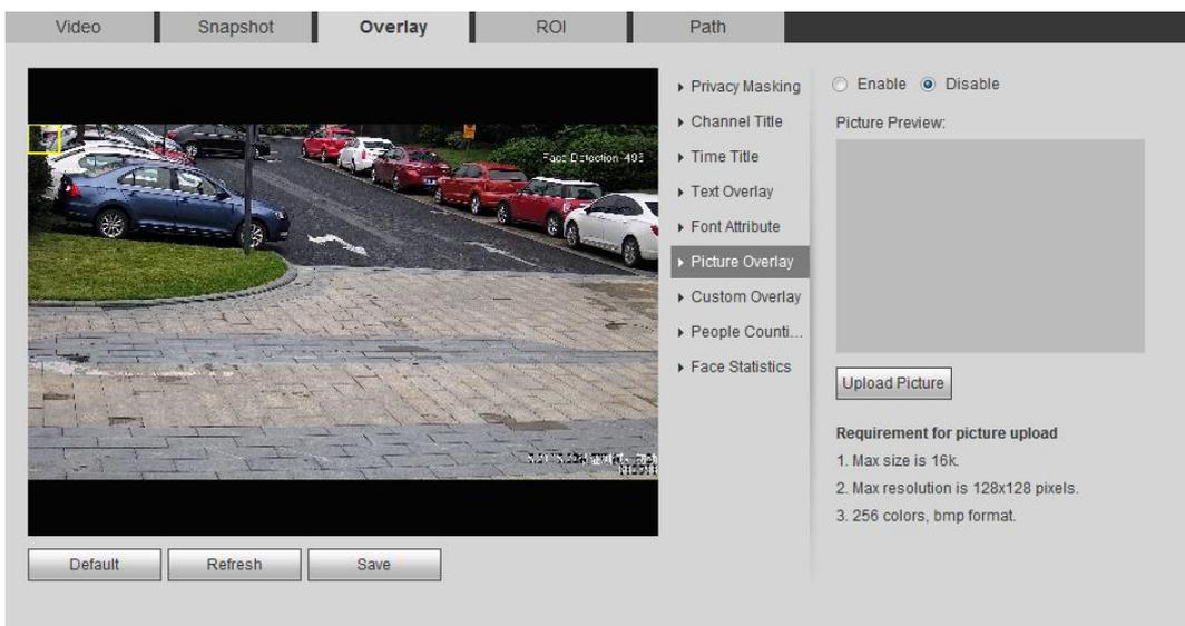
Step 2 Select the **Enable** check box, click **Upload Picture**, and then select the picture to be overlaid.
