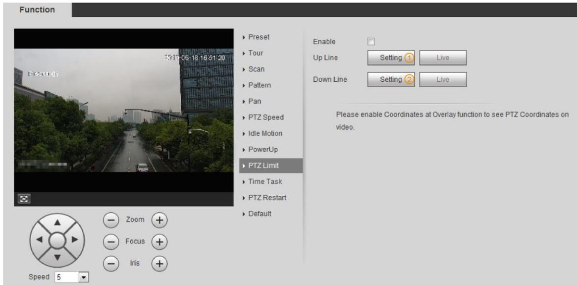
**Step 2** Control camera direction, click **Setting** ① to set up line.
