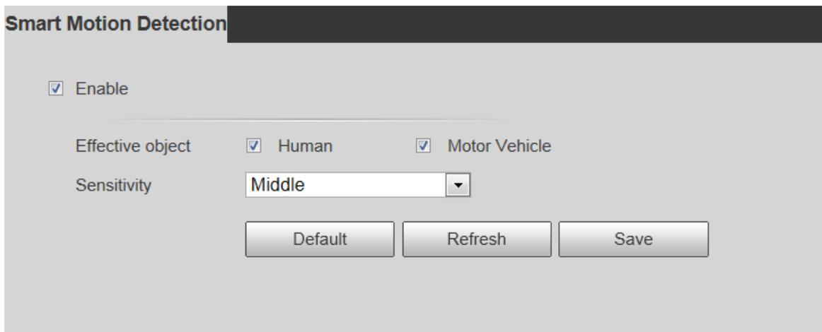
Step 2 Select the **Enable** check box to enable smart motion detection function.
