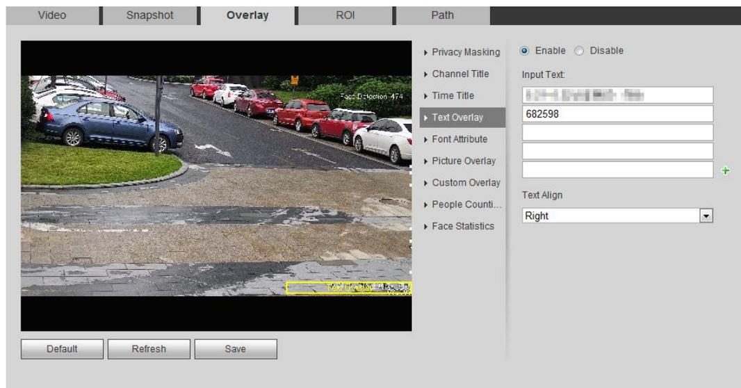
Step 2 Select the **Enable** check box, enter the text you need, and then select alignment. The text displays in the video image.
