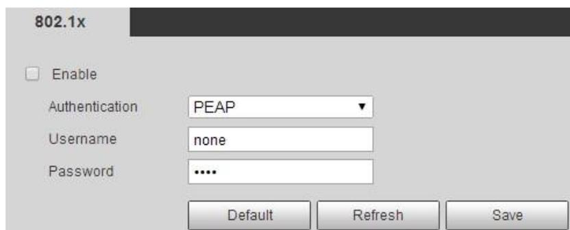
Step 2 Select the **Enable** check box, and then configure parameters. For details, see Table 4-29.
