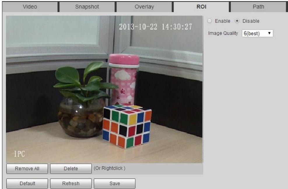
Step 2 Select the **Enable** check box, draw the area on the image, and then configure the image quality of ROI.
