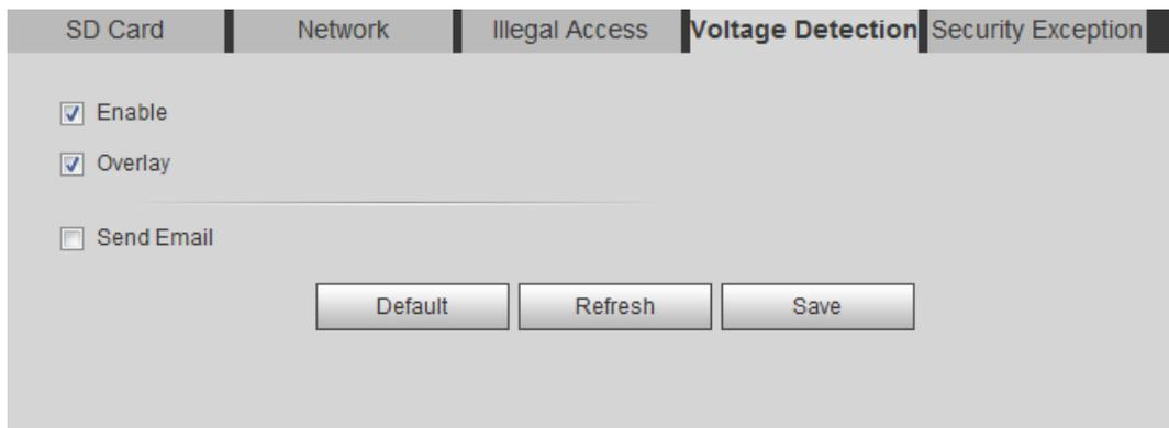
Step 2 Select **Enable** to enable voltage detection.
