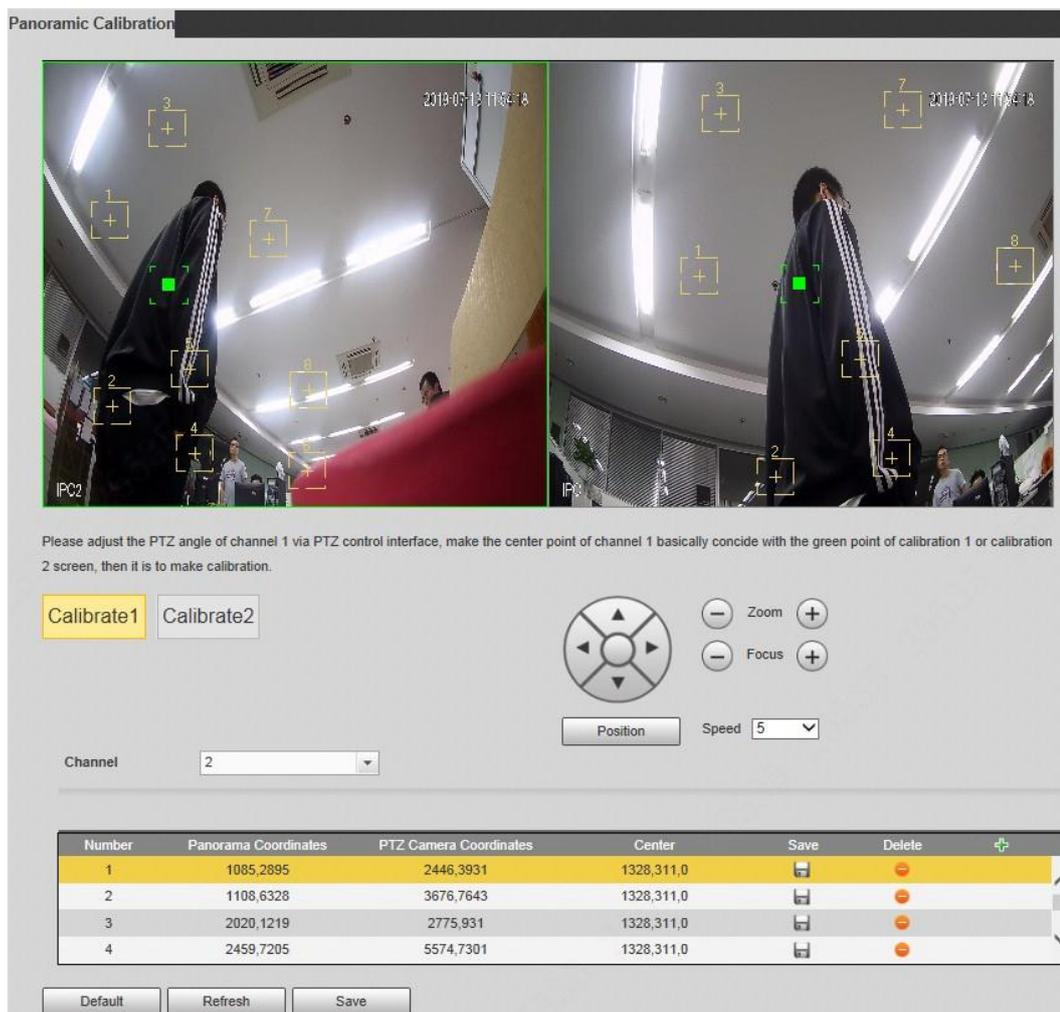
**Step 2** Select channel 2, and then select a calibration number under the video images in turns (See Figure 5-14) to add calibration points to the corresponding video images. Take **Calibrate1** as an example.
