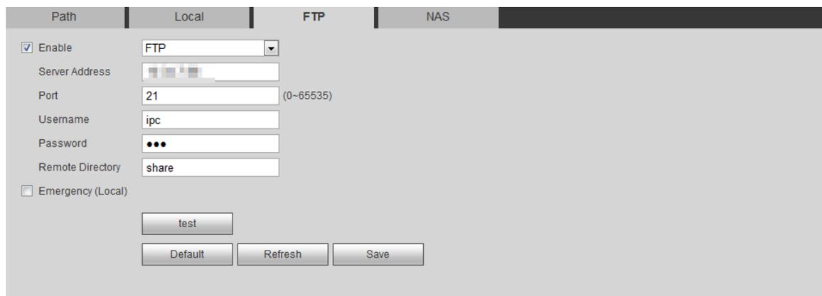
**Step 2** Select the **Enable** check box to enable FTP function.
