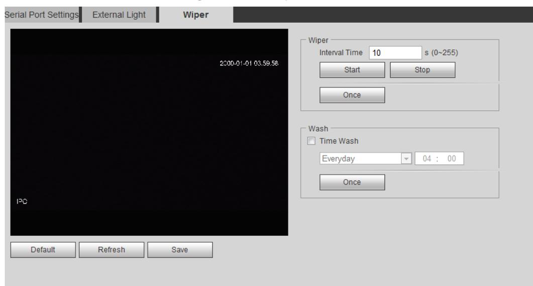
Step 3 Configure wiper work mode. For details, see Table 4-42.
