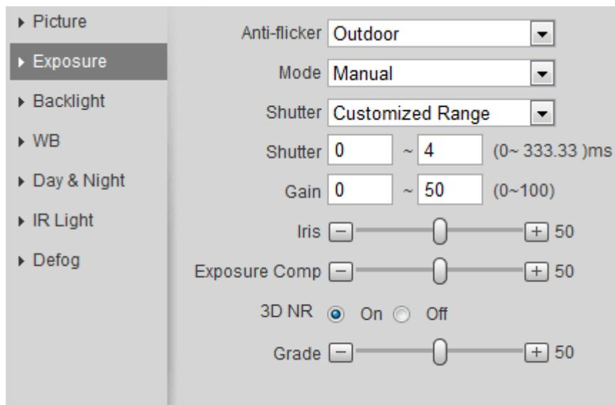
Step 2 Configure exposure parameters. For details, see Table 4-9.
