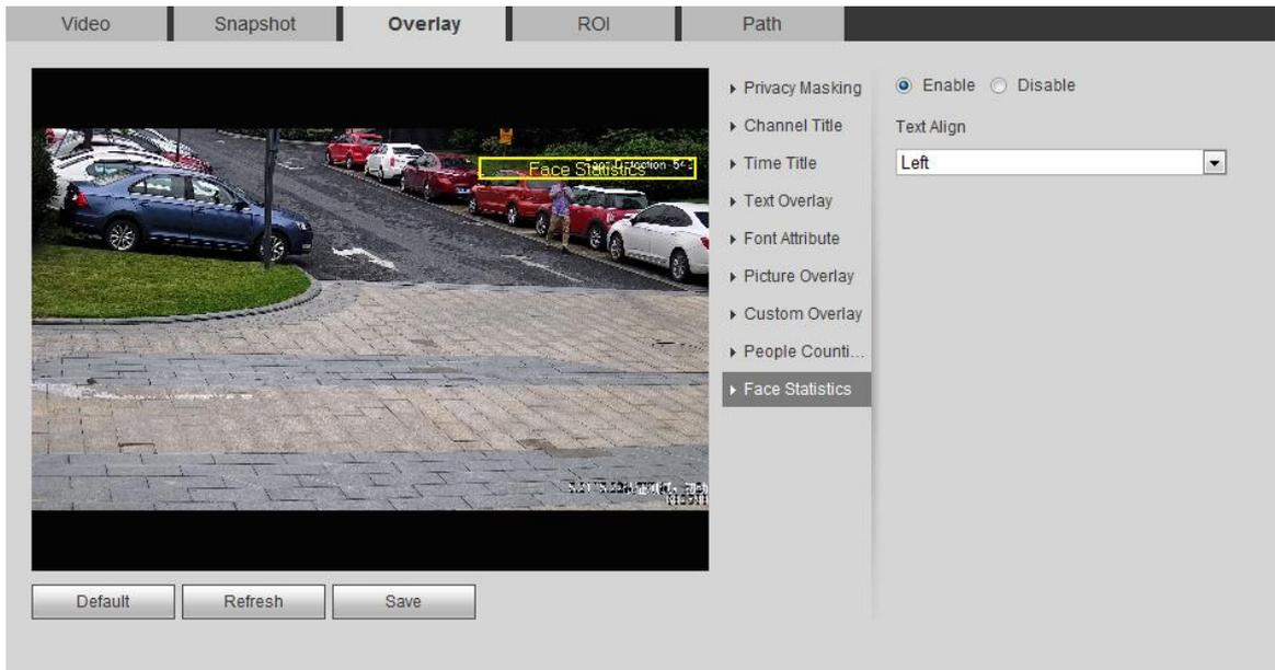
**Step 2** Select the **Enable** check box, and select the text align.
