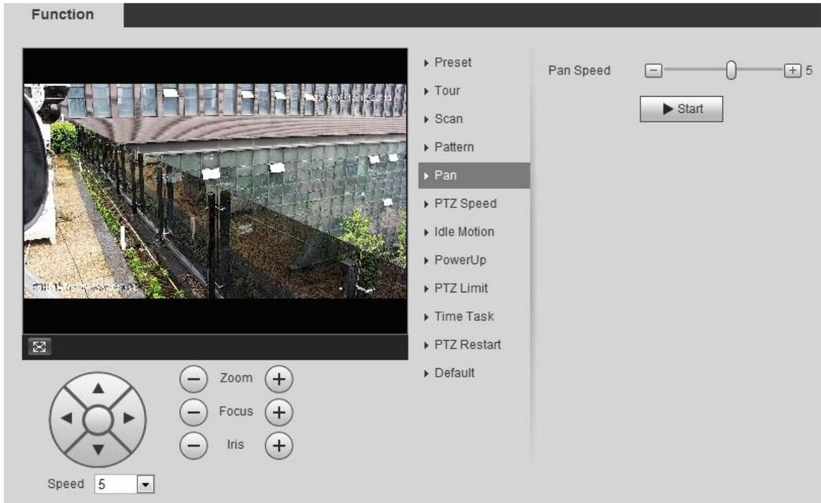
**Step 2** Set the pan speed and click **Start**, and the camera starts horizontal rotation. Click **Stop** to stop rotation.
