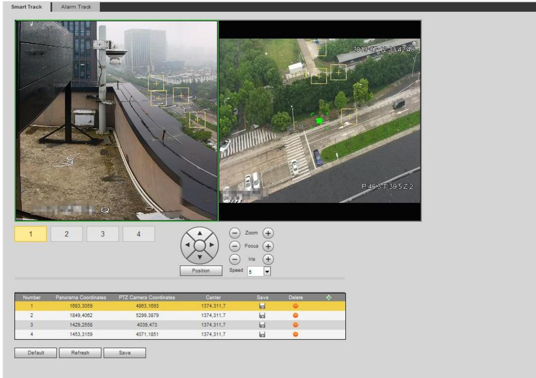
**Step 2** Select scene number under the video images in turns (See Figure 5-11) to add calibration points to the video images of the corresponding scene. Scene number 1 to 4 are four scenes divided by spliced image with at least four calibration points for each scene.
