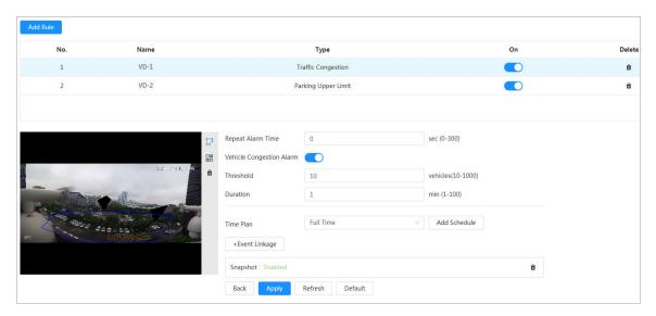
Figure 8-26 Vehicle density (parking upper limit)
