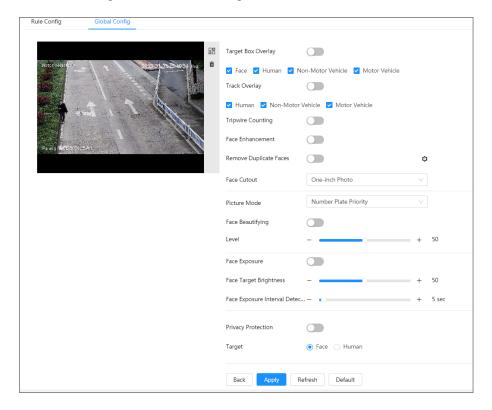
Figure 8-33 Global configuration of video metadata
