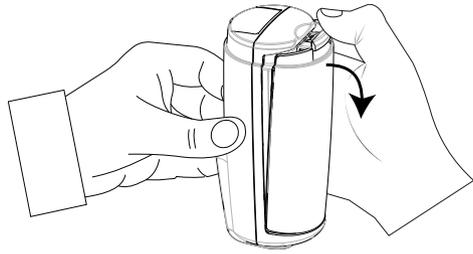
Figure 14: Opening the battery cover
