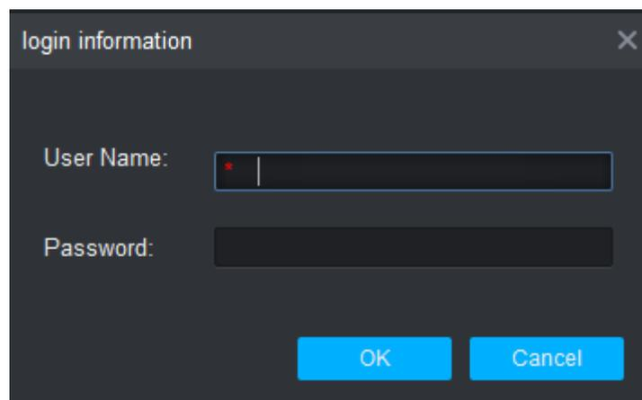
**Step 5** Input “User Name” and “Password” to log in the device, and click “OK”.
