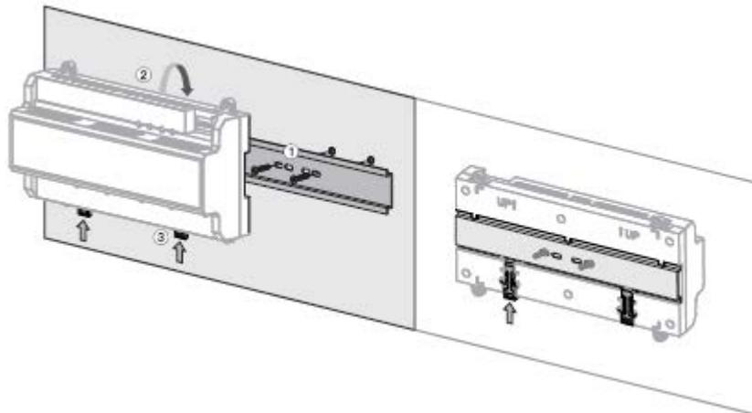
Step 1 Fix the U-shaped guide rail onto the wall with screws.
